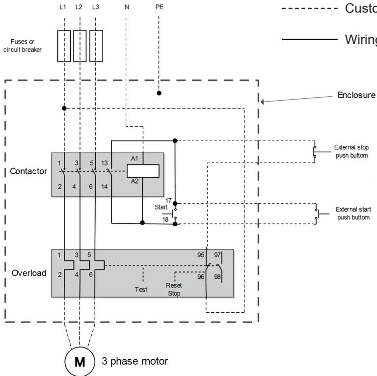
Additional start and stop stations can be wired to the DOL control circuit. In principle, the start buttons should be momentary normally open device and wired in parallel with terminals 17 & 18.
